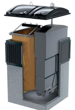
During emptying, the lid, quick lifting equipment or hinge and the lifting bag should be checked for any tears, cracks and cuts. While checking the lifting bag, special attention should be paid to the closing rope, the rope lock and the lifting loops.
